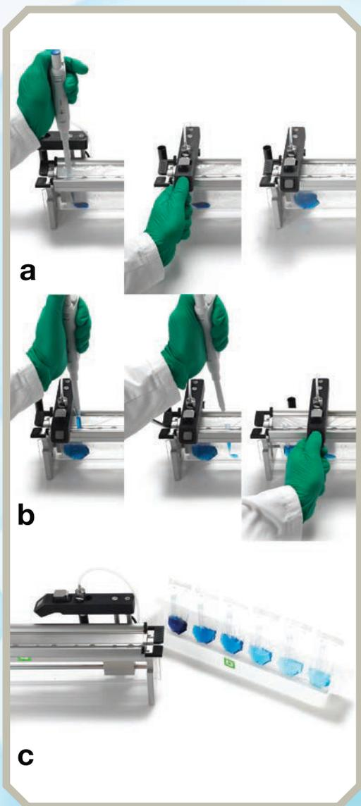
**01** Serial dilution in single-use sterile bags. A 1 ml sample together with the pipette is added into the first bag. The dosing arm is connected to the tip and the sample ten-fold diluted by adding 9 ml diluent by pressing the button (a). Diluted sample is taken out for plating and for the next dilution step (b). After finishing the serial dilution and the plating of the diluted samples used bags are removed for disposal (c). Watch video under [www.inlabtec.com](http://www.inlabtec.com)
