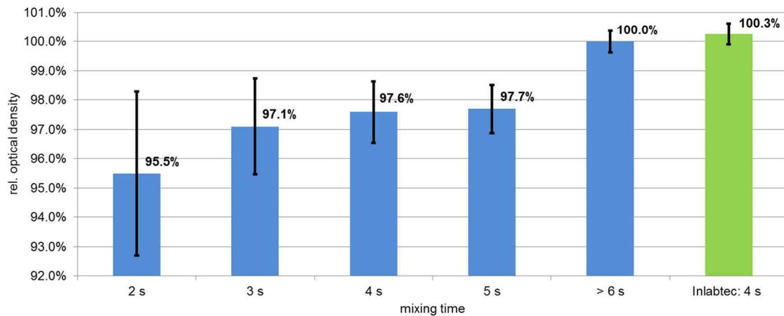
Fig. 1: Sample homogeneity as a function of mixing time measured by optical density.
