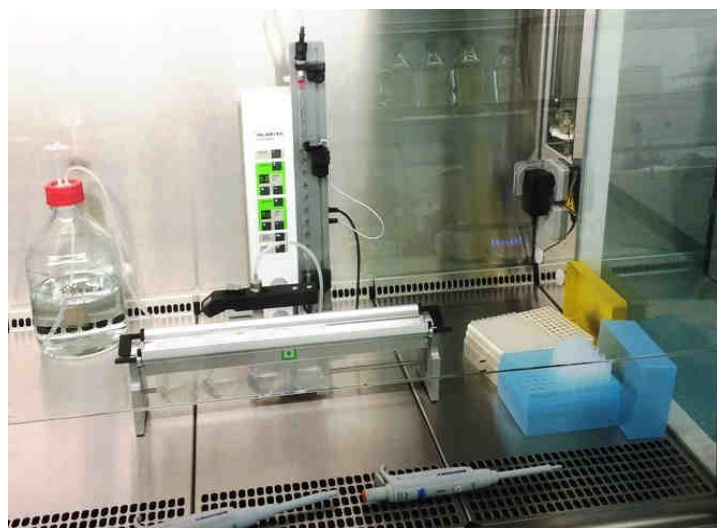
Figure 1: Inlabtec Serial Diluter installed in the clean bench of the ISO/IEC 17025 accredited and GMP compliant Swiss testing laboratory.
